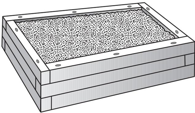
**Figure 5.** Landscape timbers make an attractive raised bed. Drill holes through the timbers to drive rebar into the ground as far as the bed extends above ground.
