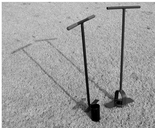
Figure 1. Use a long-handled bulb planter, or plugger, to remove soil cores before planting zoysiagrass plugs.
