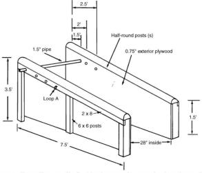
Figure 3. Breeding stall. A %-inch rope is attached to loop A, brought behind the mare above the hocks, and wrapped twice around the end of the pipe at the mare's right shoulder. The end of the rope is securely held by an attendant who can release it if necessary in an emergency.
