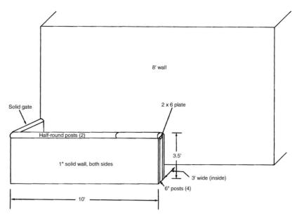
Figure 4. Teasing stall. If stall is positioned against a building, be sure the roof overhang cannot be reached by a rearing horse. A colt pen 20-30 feet in front of the mare is very desirable. It should be easy to see through but should be constructed of mesh wire small enough that a colt's feet do not go through.
