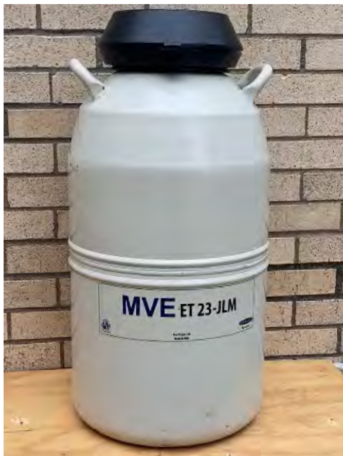
Figure 2. A liquid nitrogen tank should be stored on a wooden or composite platform rather than placed directly on an abrasive surface, such as concrete.
