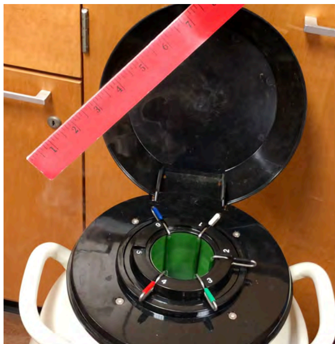
Figure 4. Measuring the level of liquid nitrogen in the tank.
