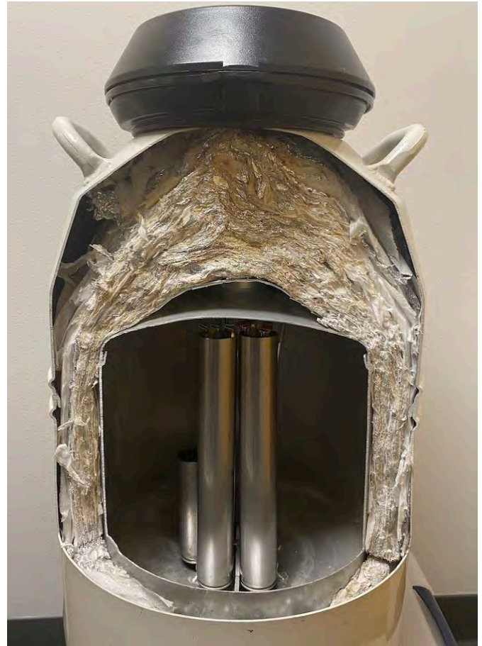
Figure 1. A cutaway tank showing the internal structure of a liquid nitrogen tank.
