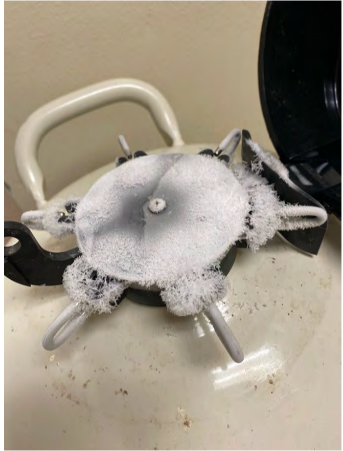
Figure 6. Frost formation on the plug, indicating a severely damaged liquid nitrogen tank.
