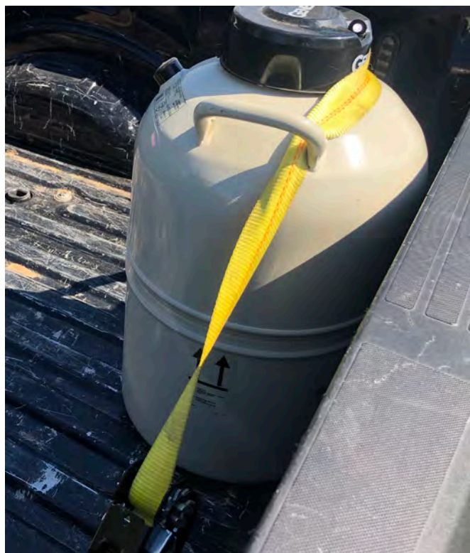
Figure 3. A liquid nitrogen tank secured in a vehicle for transportation.
