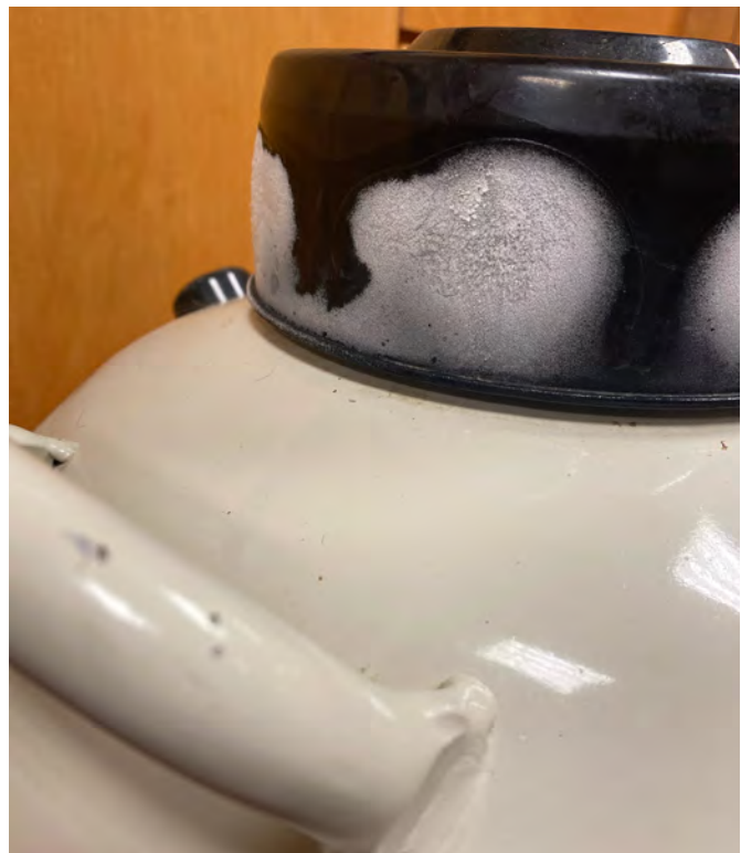
Figure 7. Frost accumulation around the lid of the tank indicate a slow to severe leak.
