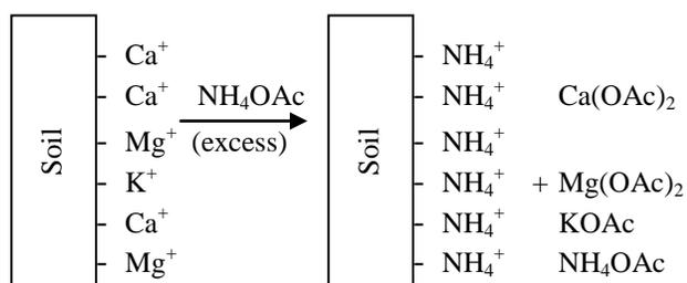
The potassium concentration in the ammonium acetate soil extract is determined by flame emission. The extract sample is sucked
