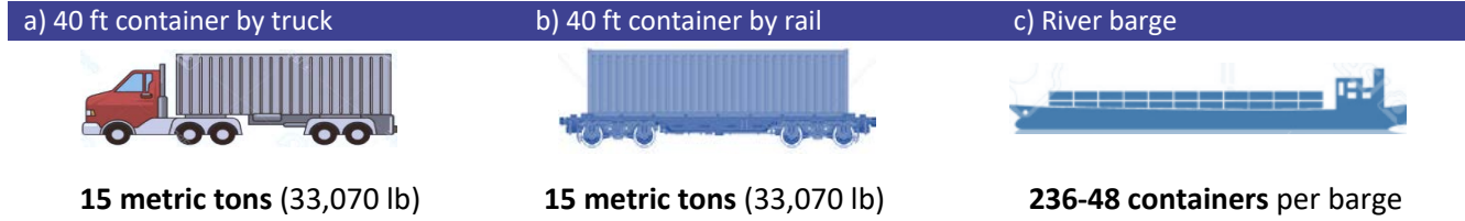
Figure 61. Unit capacity by assumed mode of transport, in metric tons and 40 ft containers.
