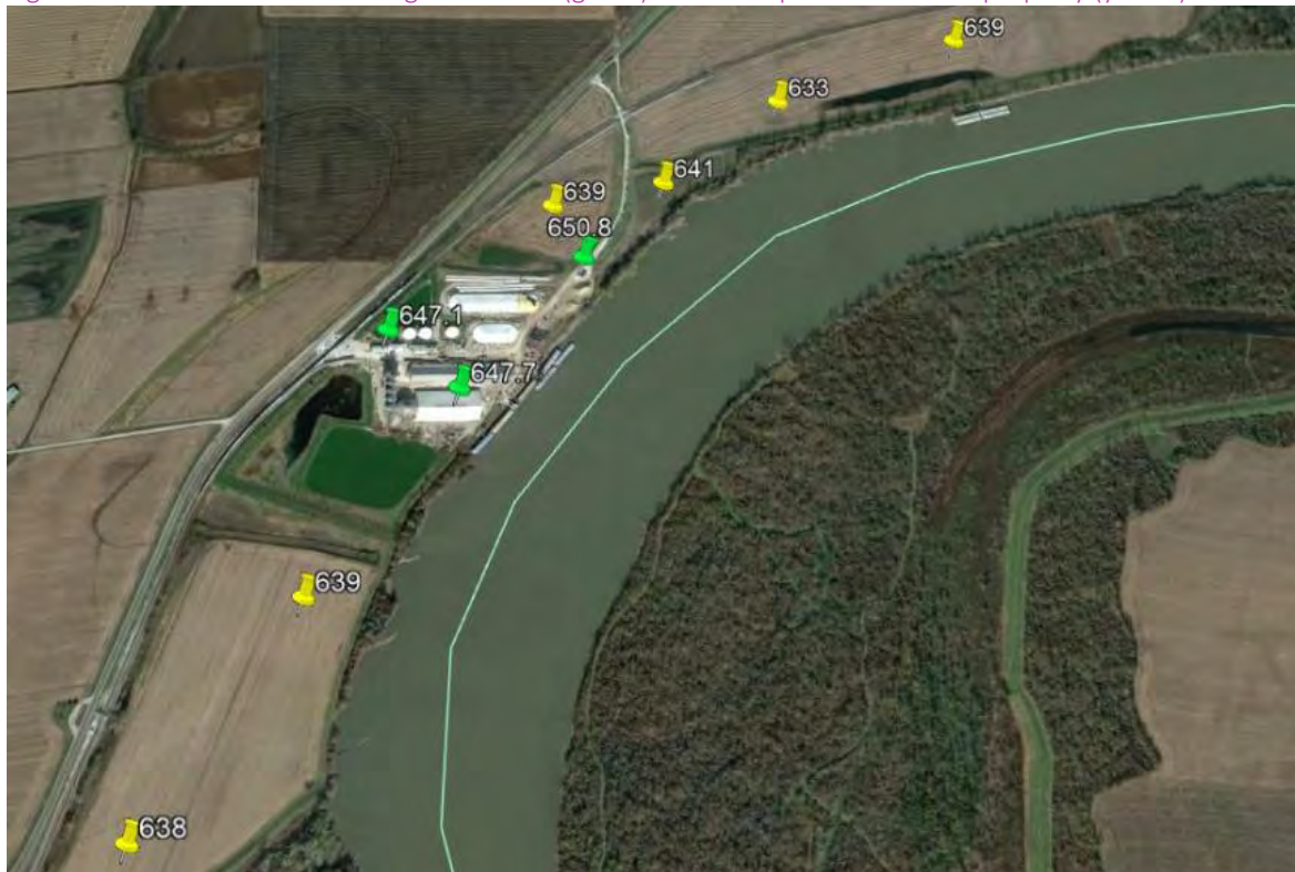
Figure 48. Elevations from building certificates (green) and other points inside the property (yellow)
