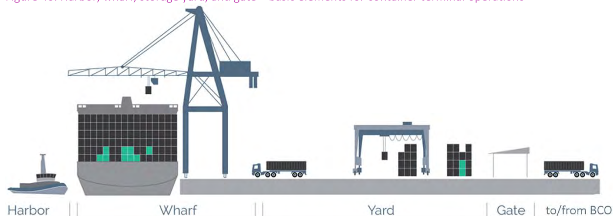
Figure 40. Harbor, wharf, storage yard, and gate—basic elements for container terminal operations
